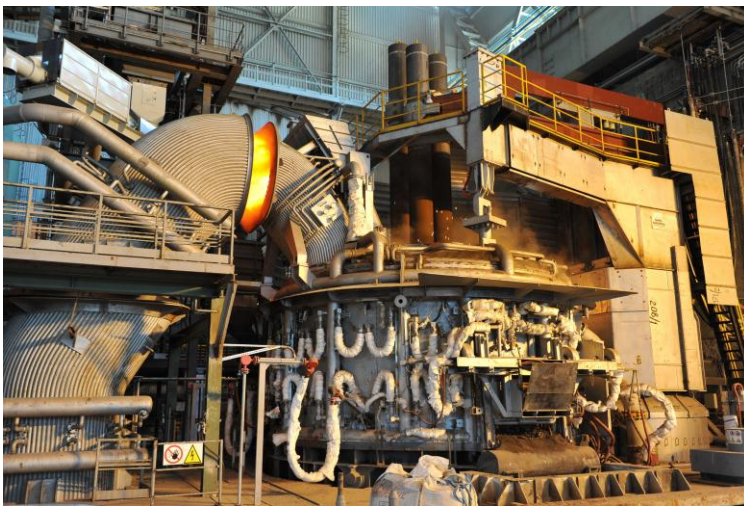
The ARCESS® electric arc furnace at the Tagmet plant.
