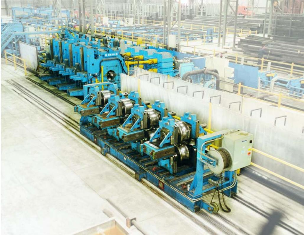
Two newly developed inside scarfers have been supplied for the 16-inch ERW line installed by SMS group in Harrow, Canada, in 2000.
