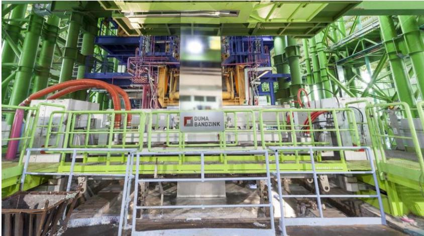
In the future, a DUMA-BANDZINK Jet-Pro air knife system will produce high-quality surfaces in the hot-dip galvanizing line No. 3 of SSAB, Finland. (The picture shows a plant of similar design).
