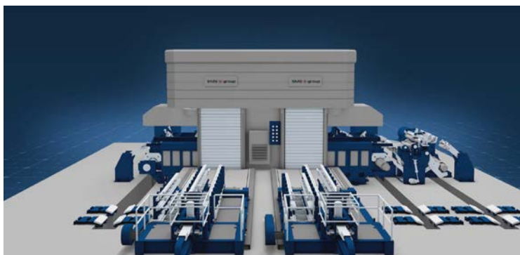
Caption: Conceptual design of a twin-stand CCM ® supplied by SMS group to Hoa Sen Group.
