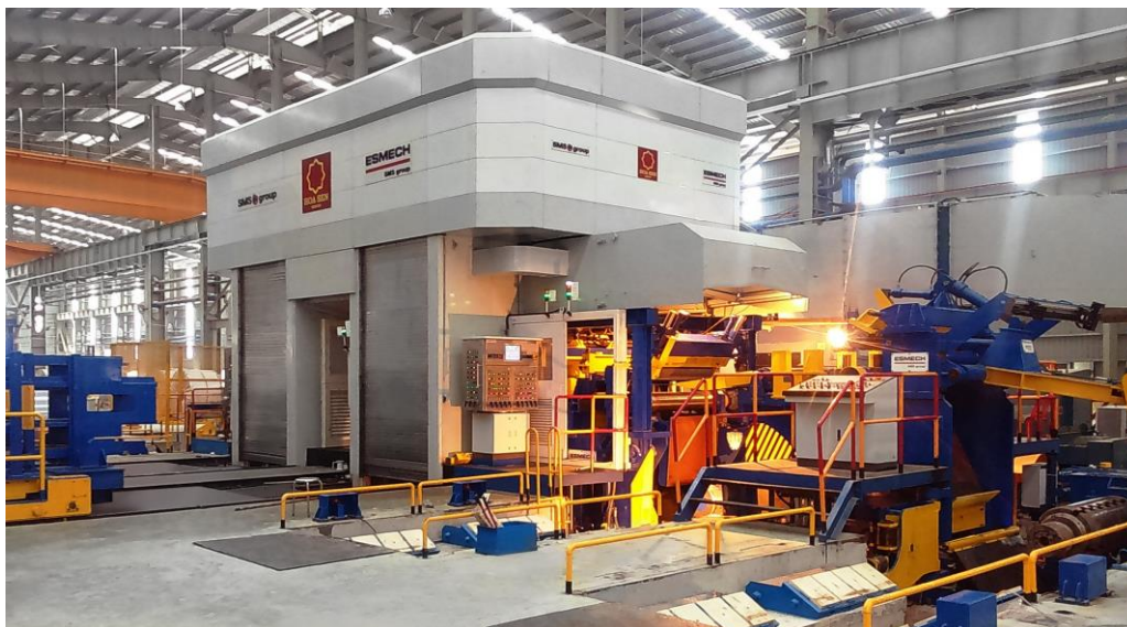
Entry section of the CCM ® equipped with pay-off reel and reversing reel No. 2.
