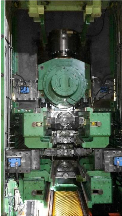
The mill stand is the centerpiece of the RCM. It is provided with hydraulic adjustment, CVC® plus roll shifting, positive and negative work and intermediate roll bending.
