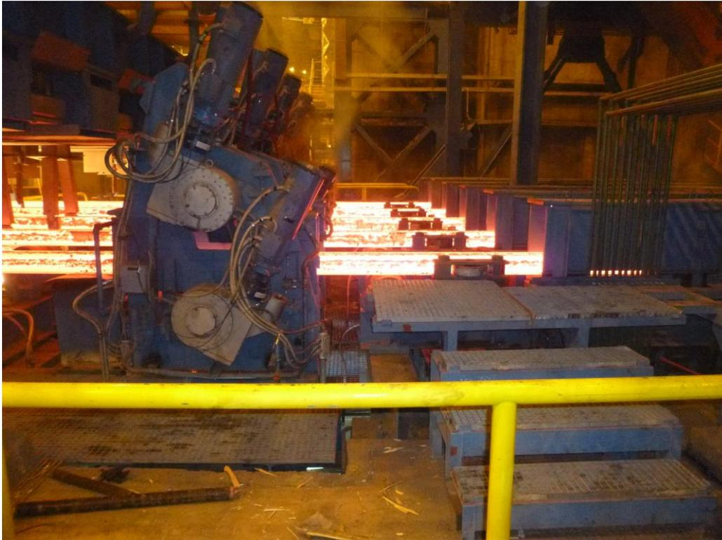
The first cast on the SMS Concast continuous billet caster.
