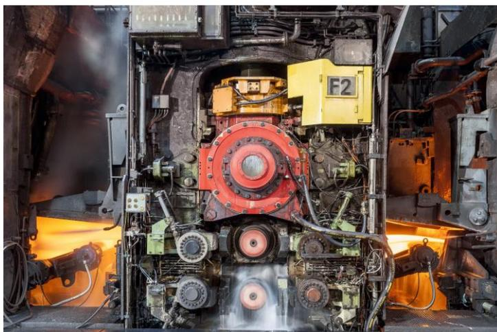
Hot strip finishing stand with subsequently installed CVC®plus system.
