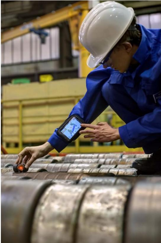
Reliable measurement of continuous caster segments and molds using the HD LASr plant assistant system from SMS group.
