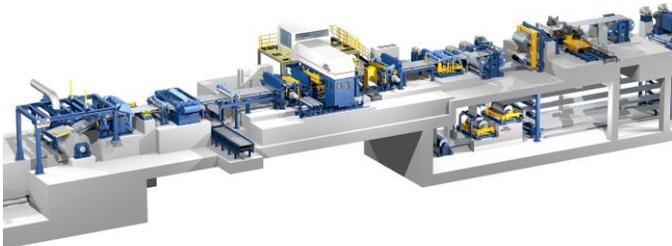
The new hot-dip galvanizing line for hot strip being built by SMS group for Wuppermann in Hungary will receive the same line entry configuration consisting of a seven-roller flattener and a side trimming unit as the one lately successfully commissioned in Moerdijk.
