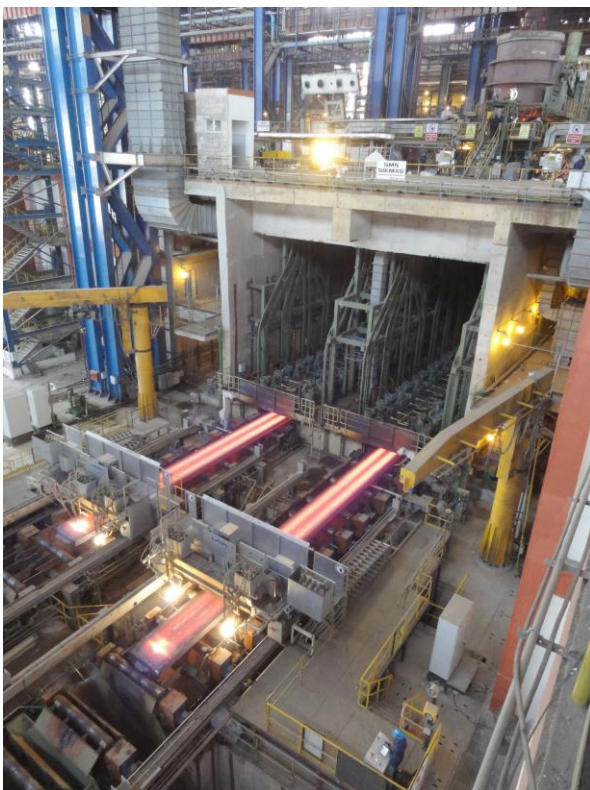
Continuous slab caster with two strands.
