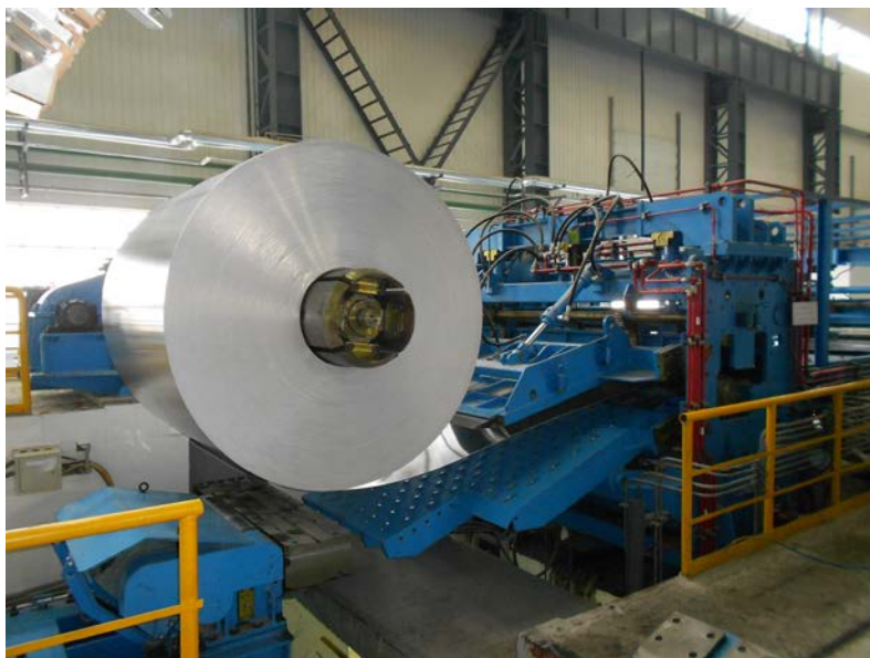
A coil being inspected in the offline inspection unit.
