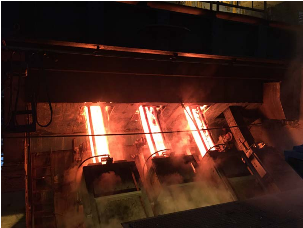
PT. Gunung Garuda successfully produces beam blanks on new four-strand caster supplied by SMS Concast.
