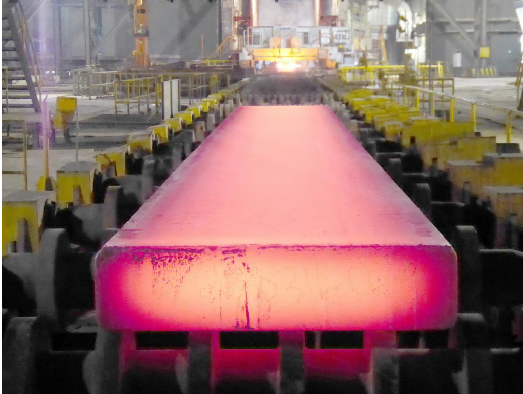
The continuous caster produces high-quality slabs.
