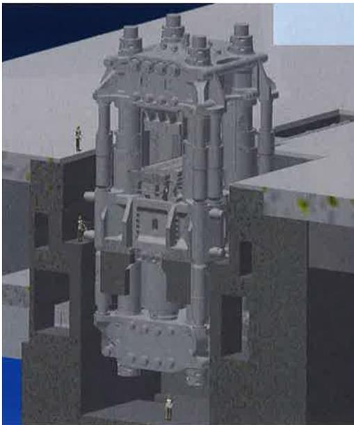
Picture illustrating the dimension of the 540-MN closed-die forging press for OTTO FUCHS.
