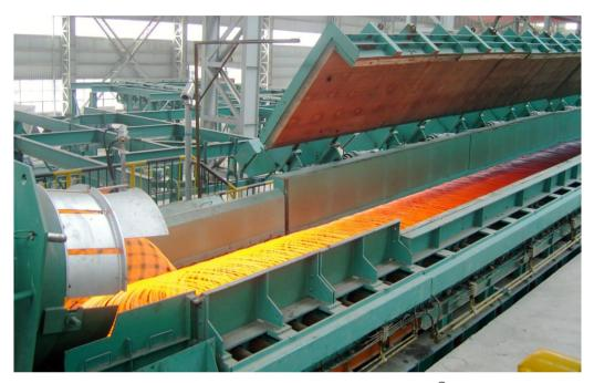
High-speed laying head and loop cooling conveyor (LCC®) of similar design from SMS group in operation in a different mill.
