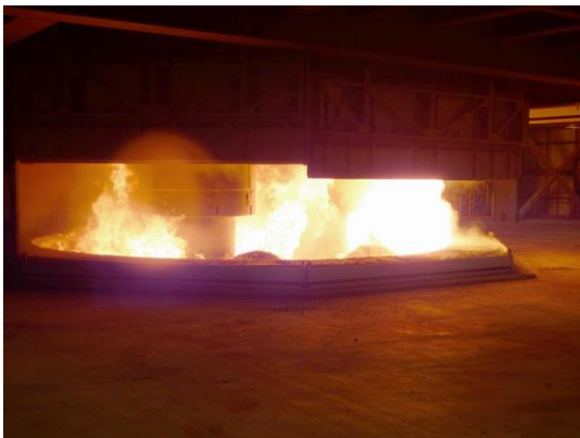
Submerged arc furnace from SMS group for the production of metallurgical silicon.
