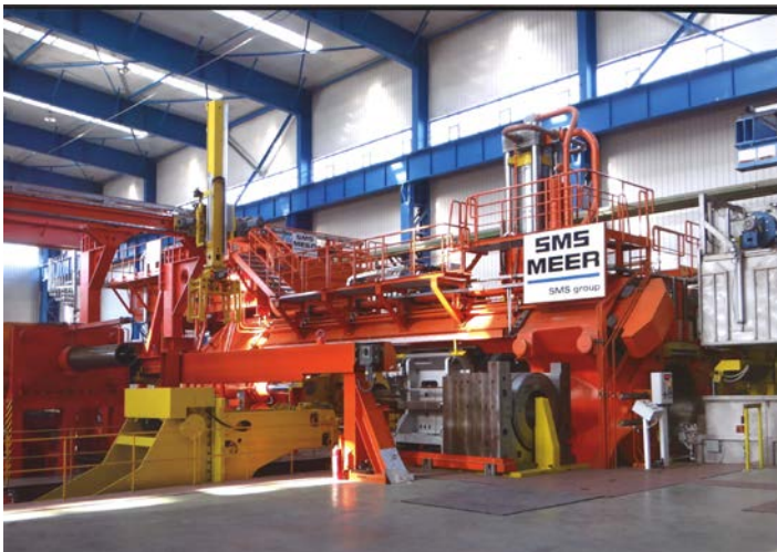
Largest front-loading extrusion press built by SMS with 160 MN press force.
