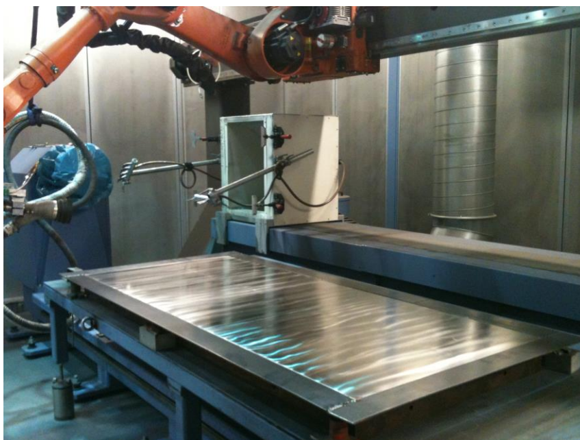
UNIGUARD™ coating of a copper mold on an HVOF machine (High Velocity Oxy-Fuel).
