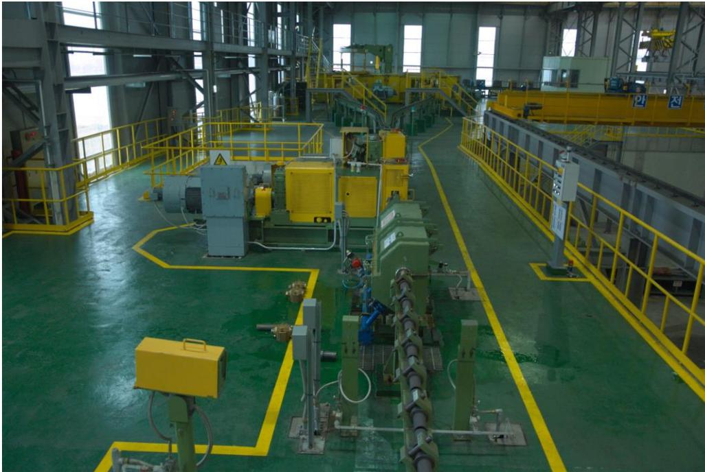
VCC<sup>®</sup>-line (Vertical Compact Coiler) at Daehan Steel Co., Ltd., in Pyeongtaek, South Korea achieves a throughput of 70 tons per hour.
