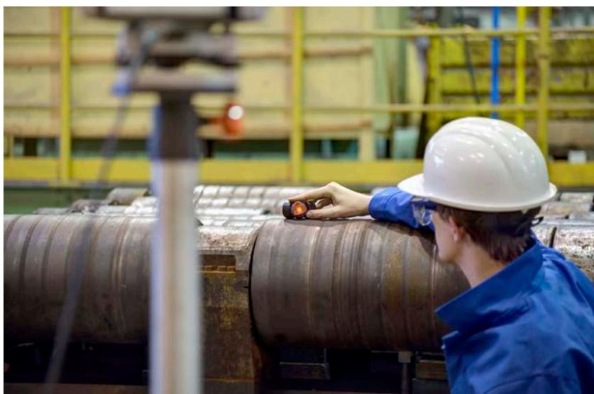
The HD LASr alignment assistant developed by SMS group provides precise measurements of the mold and the segments of continuous casting plants.
