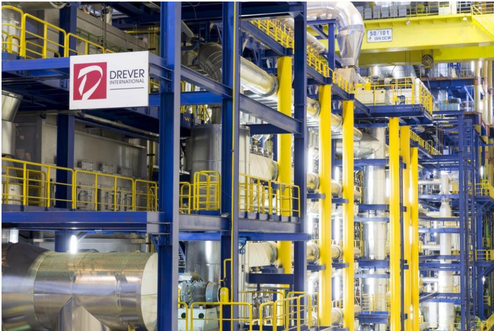
Drever radiant tube furnace in a hot-dip galvanizing line.
