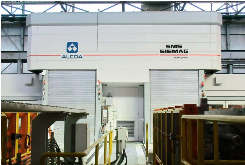
ALCOA operates the new twin-stand tandem cold mill at its Tennessee plant.
