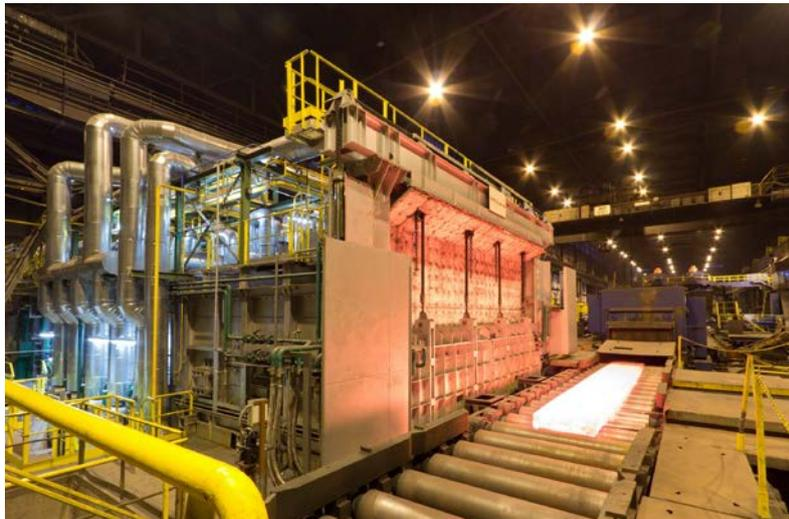
Reconstructed pusher furnace with a throughput of 90 tons per hour feeding the plate mill at VÍTKOVICE STEEL, a. s. Ostrava, Czech Republic.
