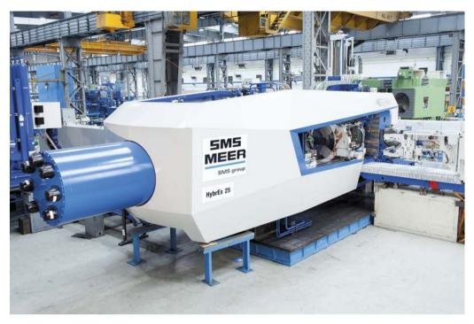
HybrEx is SMS group's latest generation of extrusion presses (in photo: The HybrEx 25). The machine enclosure ensures a high standard of safety even without additional measures.
