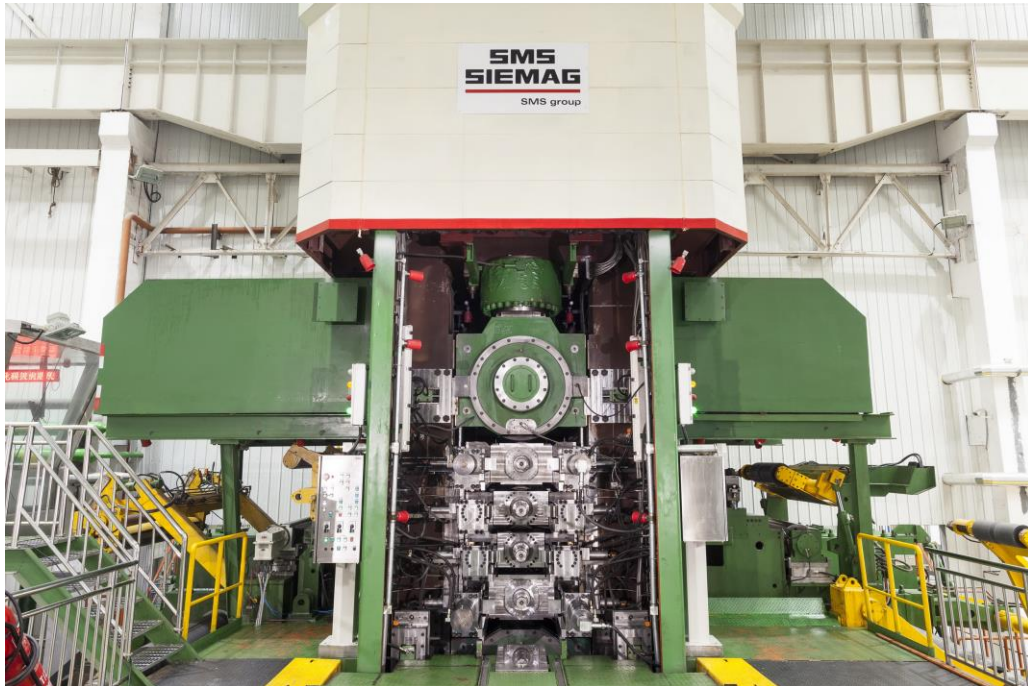
Aluminum cold rolling mill from SMS Siemag.
