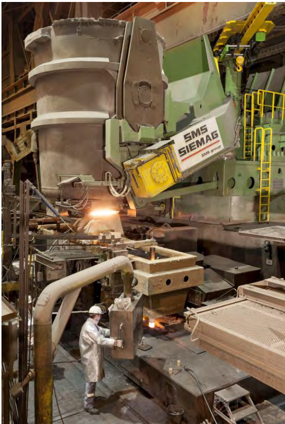
The casting floor and ladle turret of continuous caster No. 2 at Salzgitter Flachstahl GmbH's Salzgitter location.
