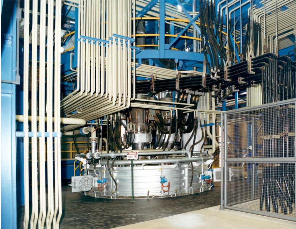
One of the submerged arc furnaces at CBMM, the SMS group supplied in 1999.
