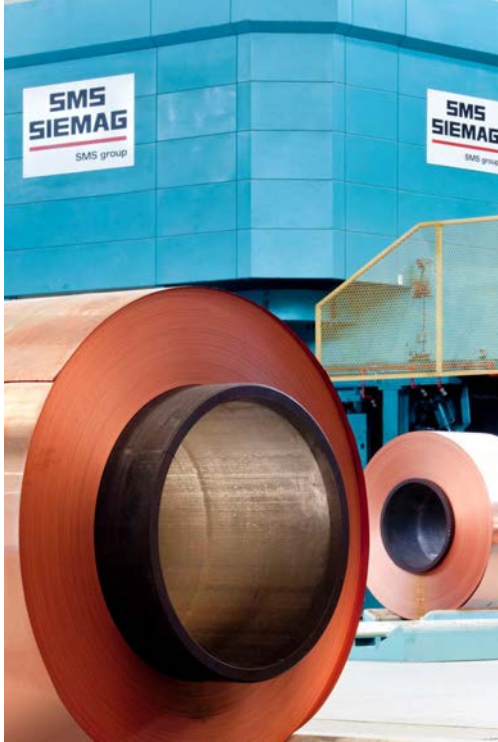
Copper strip produced on a reversing cold-rolling mill.
