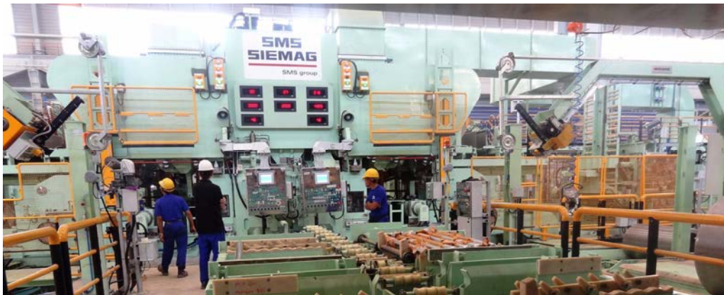
20-roll cold-rolling stand of size MB22B-52" at Bahru Stainless.
