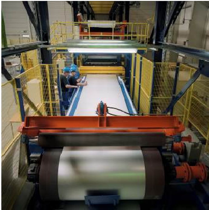
Inspection stand in the anodizing line of Coil GmbH.
